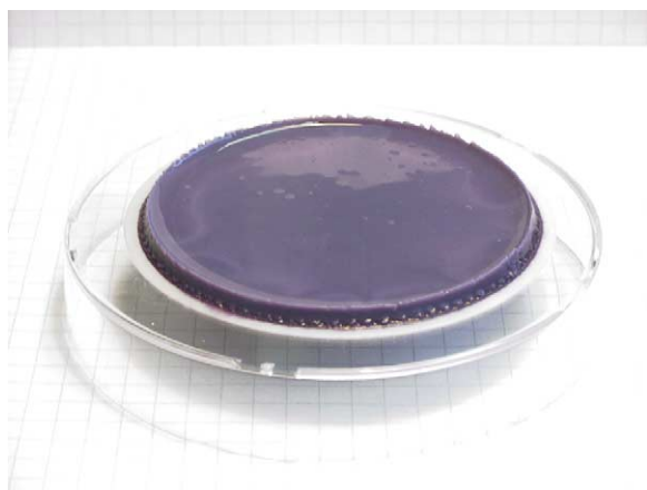
Fig. 4. Catalytically active membrane (diameter: 65 mm, thickness: 1 mm, Pd-content: 15 mg = 1 wt.%, for pore radii see Table 1).
